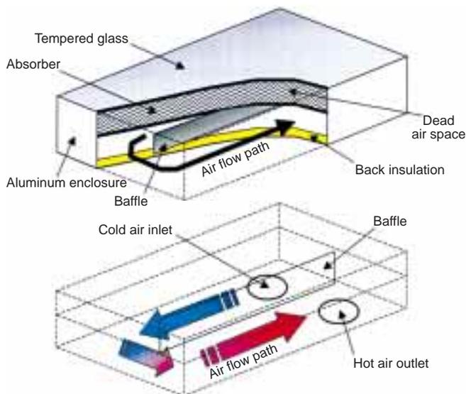
These collectors are of the single glazing/dead air space design, since some air is trapped between the absorber and the glazing. The absorber warms up when exposed to the sun, and some of this heat is transferred to the air between the absorber and the back insulation. Some absorber plates have dimples that create turbulence in the air, to better transfer heat to the air. Figure 1 shows a typical solar hot air collector of the single glazing/dead air space design.
