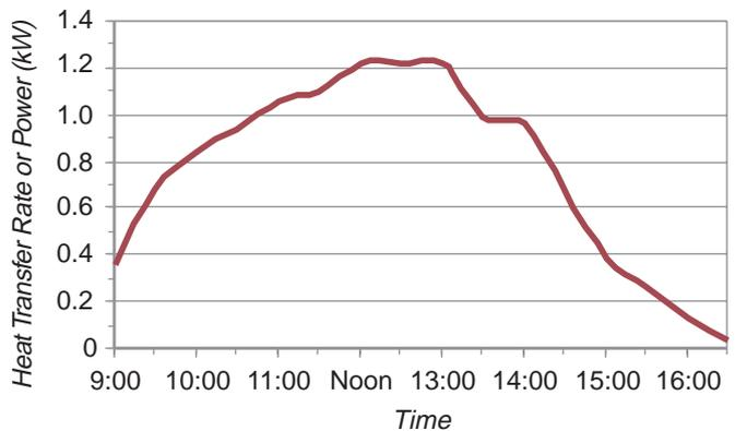
By measuring both collector inlet air temperature (T<sub>1</sub>) and collector outlet air temperature (T<sub>2</sub>) and using the above equation, the instantaneous power added by the sun through the collector to the air in the basement can be computed. The energy (kWh) can then be calculated by integrating the instantaneous power (kW) over time, in hours.
