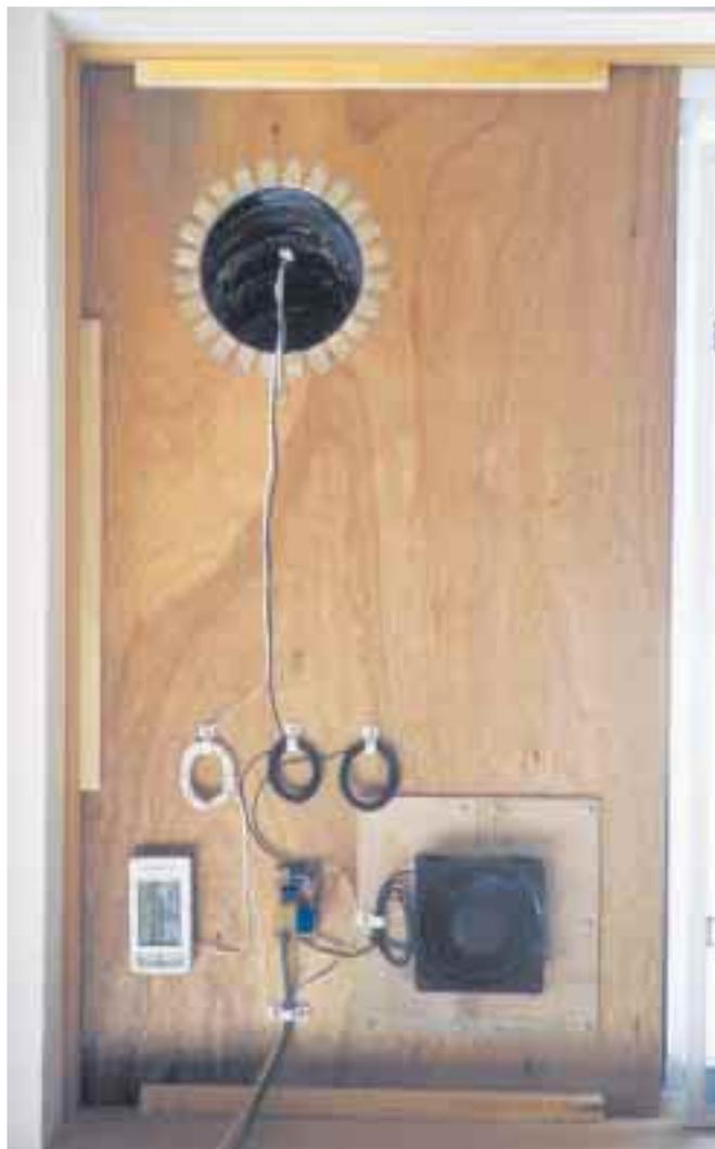
Insulated duct adapter panel, showing the fan in front of the cold air inlet (lower right), the hot air outlet (upper left), the temperature control circuit, and the dual thermometer.
