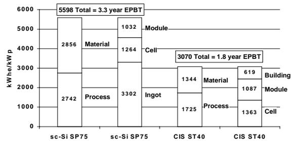
Figure 4: Energy requirements breakdown. EPBT computed at 1700 kWh/m<sup>2</sup>/year.
